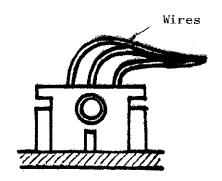
It is important to give slack to the wires of the portion, leading out of connector housing as shown above.
