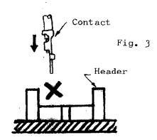
When to mount spring header onto printed circuit board, apply the header on PCB flatly, and press the middle part of the header with the fingers, so that it will fit closely over the PCB.
