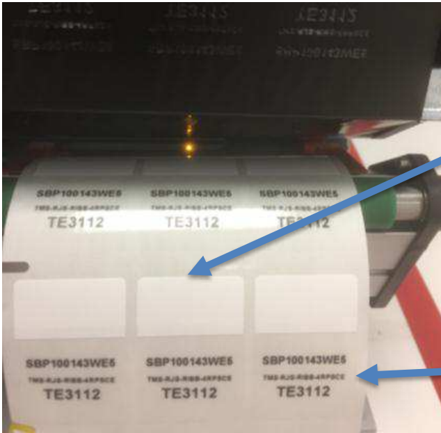
Figure 9, sensor not adjusted to side notch
