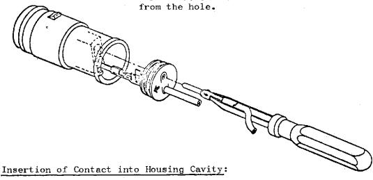
When to insert contact into housing cavity, it is important to have contact bottom facing to inside wall of corner-cut side of the cavity as shown in the figure below. With the contact bottom facing to the cavity wall, slide the contact as far as it goes until it bottms in the cavity. When the contact reaches the bottom, a small clicking sound is heard, and the contact becomes secured in position. Make sure by pulling back the wire slightly if the contact is locked in position.
