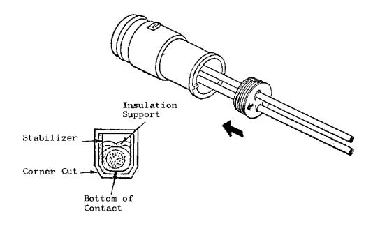
First, have the arrow marking of rubber plug set aligned with a tiny projection on the edge of housing entry opening to obtain the correct orientation. Draw circumferential edges of rubber plug through the edge of housing entry, and insert it by pressing evenly to make a uniform sink in the housing. The upper surface of rubber plug must be flush with the edge of housing, or higher than it within lmm.
