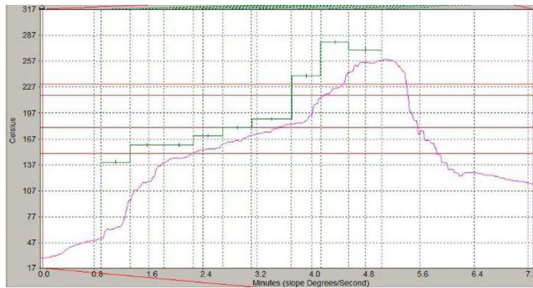
Figure 8 – Resistance to Reflow Soldering Heat – Reflow Profile
