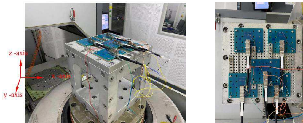
Figure 3 – Random Vibration Test Setup
