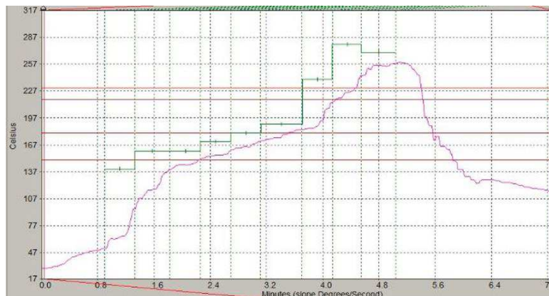
Figure 5 – Solderability Test Setup - Reflow Profile
