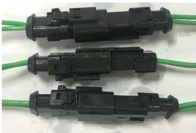
Diesel fuel RM-903/T-Xylene +60°C
