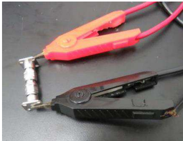
Figure 1 – Typical LLCR Setup, Center Contact
