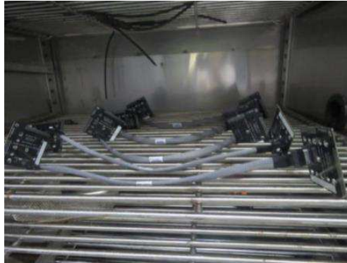
Figure 10 – Damp Heat Steady State Test Setup
