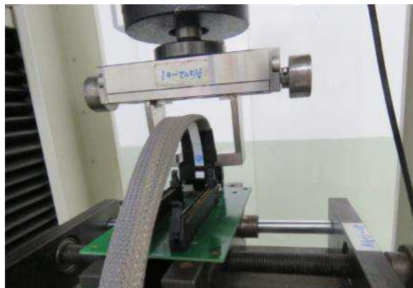
Figure 6 – Mating Force Test Setup
