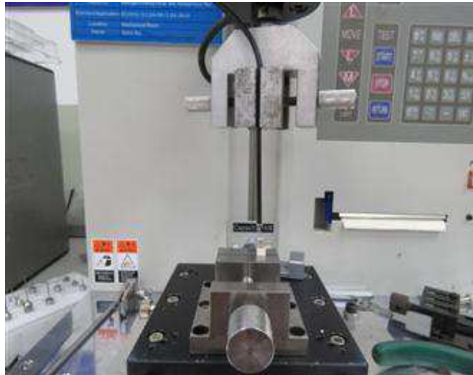
Figure – 6 typical retention force setups
