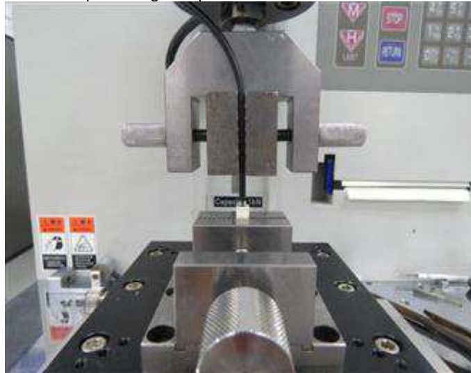
Figure 5 – typical contact insertion force setup
