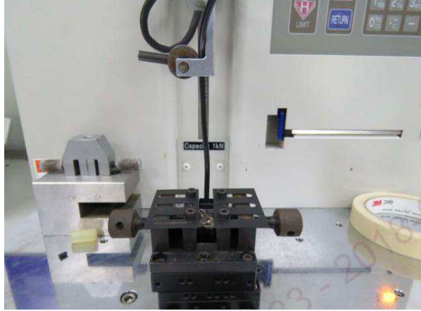
Figure – 7 typical retention force setups
