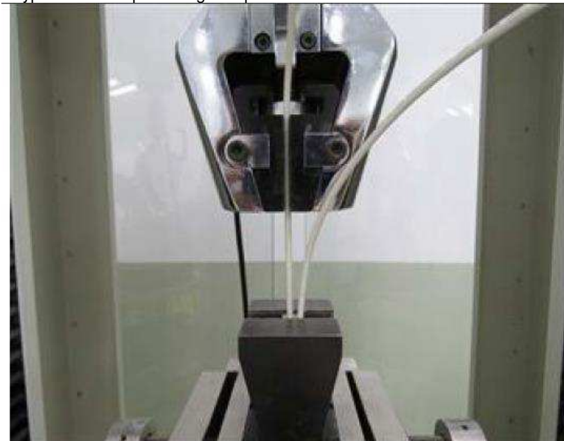
Figure 2 – typical contact insertion force setup
