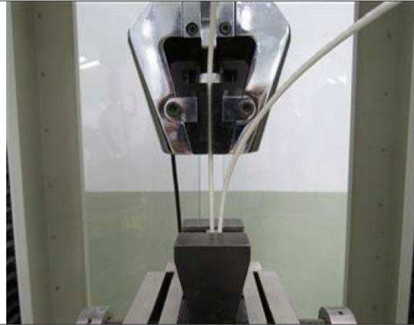
Figure – 3 typical retention force setups
