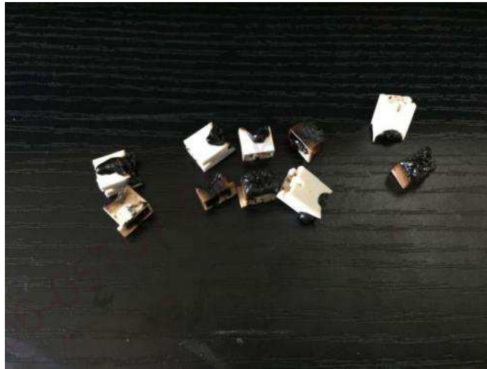
Figure 1 – visual check for after GWT 750°C test
