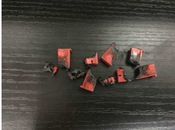
Figure 3 – visual check for after GWT 750°C test
