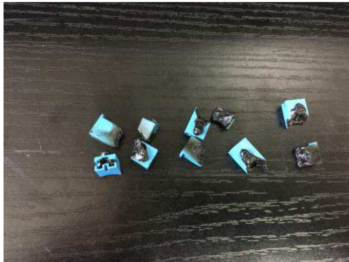
Figure 2 – visual check for after GWT 750°C test
