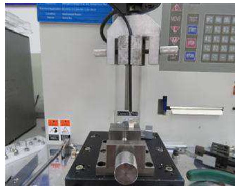
Figure – 5 retention force test set up
