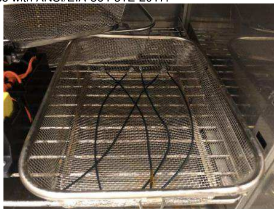
Figure - 8 test set up for humidity and temperature test
