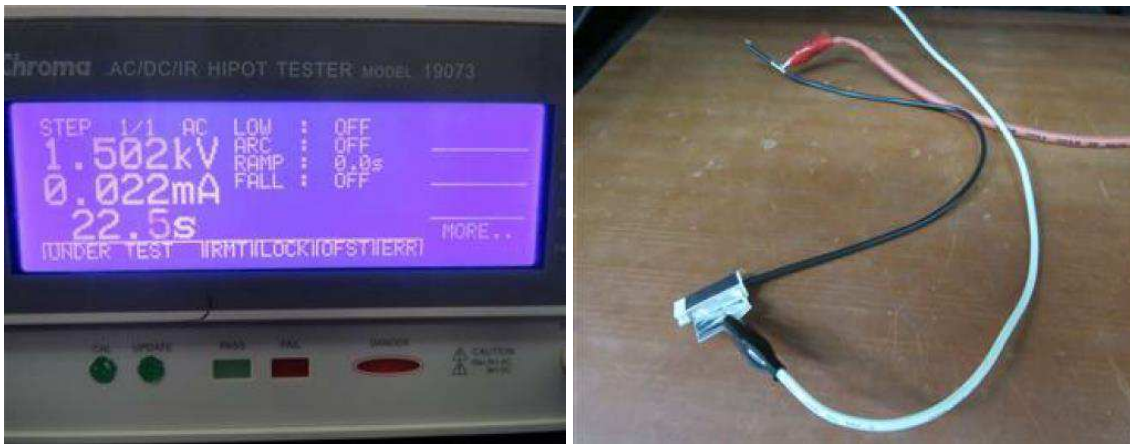
Figure - 11 typical Dielectric strength test setup
