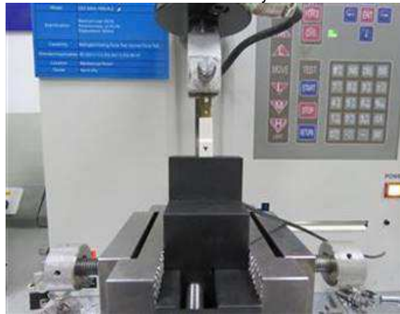
Figure – 7 Mating/Unmating test set up
