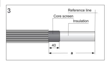
Measure the conductor bore depth of the connector and remove the insulation on both cores equal to the insert depth I (see Table 1).
