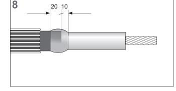
Slide the stress control tube (black) over the plastic cable core level with the end of the insulation cut back. Shrink down starting from the insulation cut back towards the oversheath as shown in the drawing.
