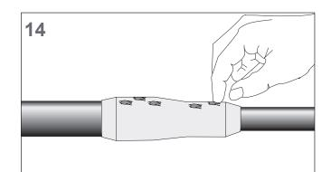
Open the large aluminium foil bag. Take out the long yellow void filling strips. Remove one release paper from the void filling tape (yellow) and roll it up.
