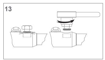
Smooth out any sharp edges of protruding bolts where appropriate. Clean and degrease the connector area and the insulation with a cleaning wipe.
