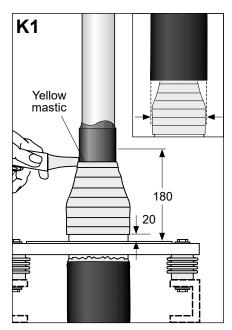
Wrap one layer of yellow mastic with an overlap of 50% onto the cable. Stretch the tape by 50% during wrapping. Wrap the mastic starting 20 mm from the base plate to 180 mm above the base plate (see drawing).
