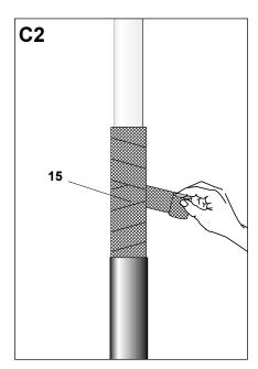
Remove the outer jacket (**110**) and bedding 100 mm below the lower mark (**LM**).
