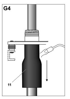
The tube is fully shrunk when the outer surface is smooth, has a glossy appearance and a flow of sealant is visible at each open end. Intimate surface contact should be made along the whole tube length, conforming to the profile of the components underneath. The tubing should be smooth and wrinkle free.
