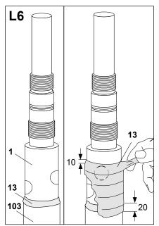
Fill the gap between the lug (1) and the cable insulation (103) with yellow mastic tape (13).
