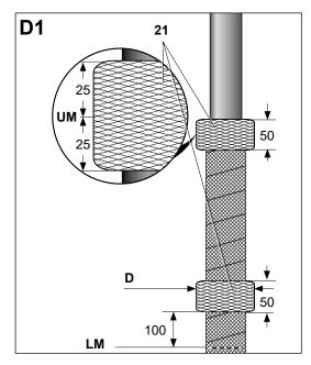
Apply a 50 mm wide packing of textile tape (**21**) on the upper mark as shown. 100 mm above the lower mark, wrap a second 50 mm wide packing of textile tape starting as shown.
