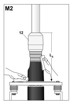
Remove the protection materials from the stress cone (**12**).
