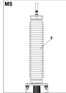
Carefully slide the composite insulator (5) over the cable assembly, the larger bottom flange first.
