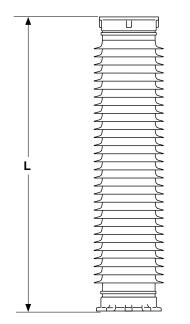
Measure the length L of the insulator (5) as shown.
