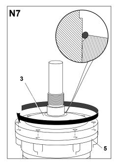
Screw the top plate (**3**) and sealing ring down until the top plate touches the flange of the composite insulator (**5**). Turn the top plate one more turn. Make sure its holes are in line with the holes of the composite insulator. Grease the O-ring.
