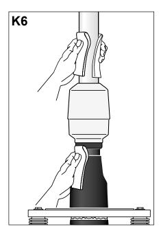
Clean the cable and all parts installed.
