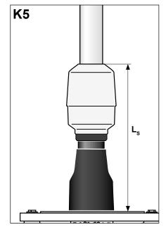
Push the stress cone with a twisting movement until its collar reaches the mark on the outer semicon layer.
