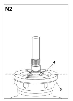
Adjust the support nut (4) temporarily so its surface **is flush with** the top of the composite insulator (5).
