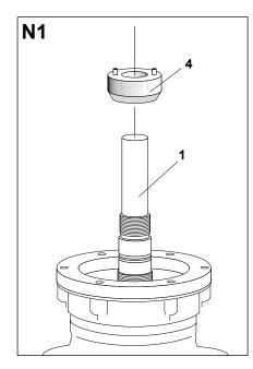
Grease the support nut (**4**) with silicone grease. Slide the support nut over the lug (**1**).
