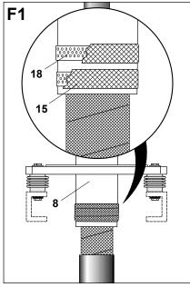
Abrade, degrease and clean the cable outer jacket (**110**), the cable gland (**8**) and the Al-tape (**107**).
