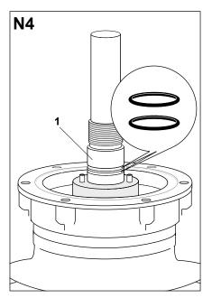
Place the sealing ring in the groove of the housing flange. Grease the O-rings with silicone grease.
