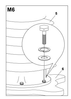
Grease the bolts with grease. Fix the composite insulator (5) to the base plate (6) as shown. Tighten the bolts cross-wise (see detail).
