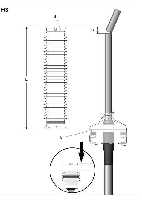
Measure the height L of the composite insulator (5).
