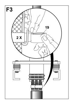
Connect the lower ends of the copper braids (24) to the Al-tape with a roll spring (19). Apply two turns of the roll spring, bend back the copper braids, then apply the rest of the roll spring.
