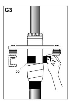
Wrap 1 layer of black mastic (**22**) around the gland above the textile tape.
