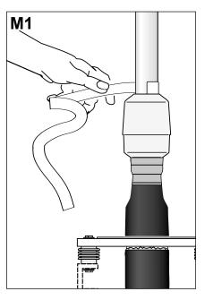
Remove the transparent tape from above the stress cone.
