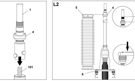
Remove the PVC tape from the conductor (**101**).
