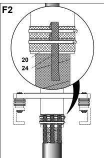
Remove the PVC tape. Fix the three copper braids (24) to the shield wires as shown using two armour clamps (20).
