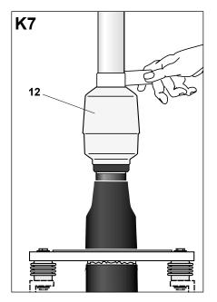
Wrap all silicone tape with an overlap of 50% onto the heat-shrink tube, the cable and stress cone.
