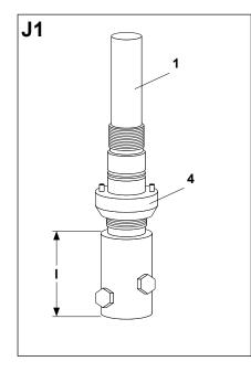
Measure the bottom part I of the cable lug as shown.
