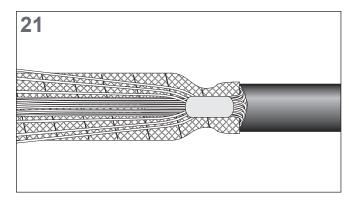
Wrap a second layer of copper mesh round the joint with a 50% overlap. Cover the complete joint area including the mechanical shield connector.
