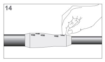
Open the large aluminium foil bag. Take out the long yellow void filling strips. Remove one release paper from the void filling tape (yellow) and roll it up.
