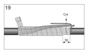
Form an earth lead of the shield wires and insert both ends into the mechanical shield connector supplied.
