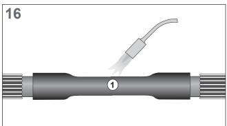
Position the screened insulating sleeve (black and red) centrally over the connector area.
