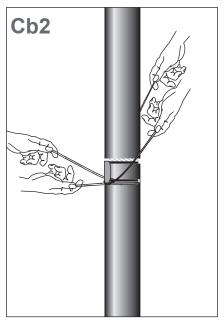
Cut through the outer jacket (110) with the supplied string. Remove the outer jacket from the metal foil (106) by slicing segments away with the string as shown in the picture.
