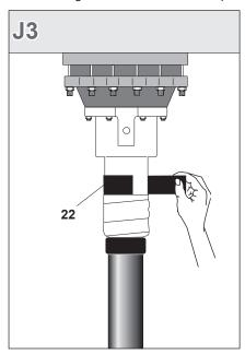
Position the heat shrinkable thick wall tubing (11) approx. 100 mm on the gland stud and shrink it into place. Start shrinking at the top then move downwards.
