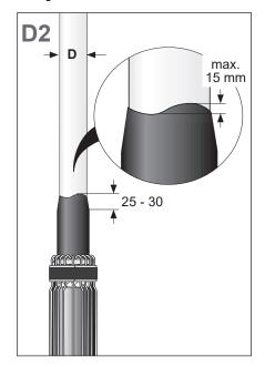
**Chamfer the outer semicon layer** in between 25 to 30 mm.
