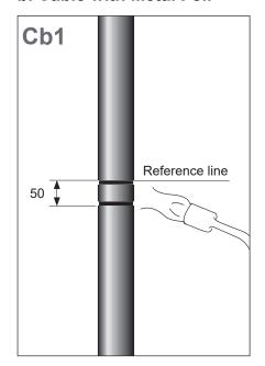
Heat the cable outer jacket (**110**) below the reference line. Soften approx. 50 mm of the surface.
