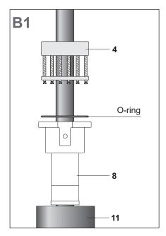
Move the heat shrinkable thick wall tubing (11), cable gland (8) and O-ring down the cable jacket as shown in the drawing.
