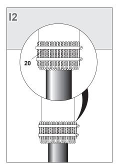
Cut the shield wires and bend them back onto the cable gland. Fix the shield wires as shown using two armour clamps (20).
