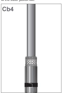
Install the roll spring (19) around the shield wires. Tighten the roll spring with a twisting action. Remove the wire binder which is near the cable oversheath.
