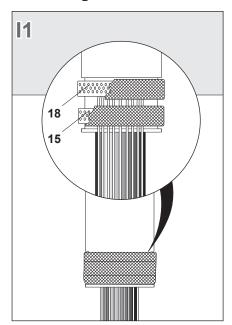
Abrade, degrease and clean the cable outer jacket and the cable gland.
