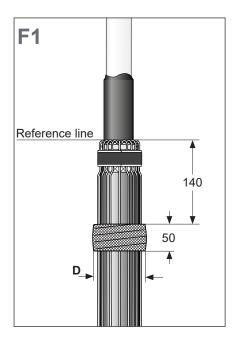
**140 mm below the reference line,** apply a 50 mm wide packing of cotton cloth tape.
