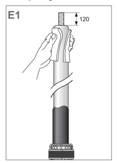
Remove 120 mm of the cable insulation (103) as shown.
