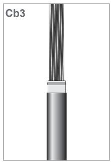
Fix the metal foil (106) with a wire binder. Clean the metal foil from traces of the outer jacket (if any). Remove the outer jacket, foil and bedding from the remaining cable end.
