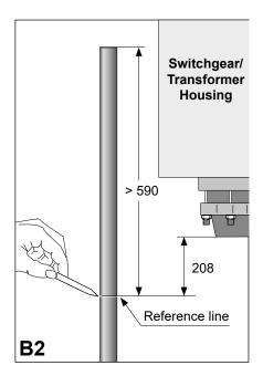
Mark the reference line on the cable 208 mm below the transformer housing as shown.
