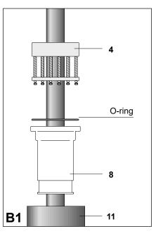
Move the heat shrinkable thick wall tubing (11), cable gland (8), O-ring and compression device (4) down the cable jacket as shown in the drawing.
