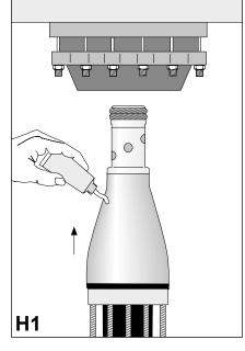
Remove the temporary protection from the connector stud. Clean and degrease the gray cover part of the silicone stress cone (**12**) with alcohol.
