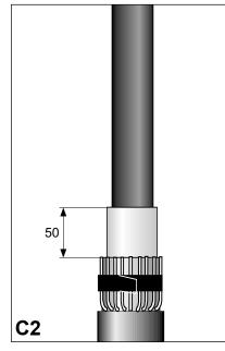
Remove the copper tape screen to within 50 mm from the AI wire armour cut.
