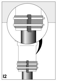
Pull the Al-wires out of the cable gland.
