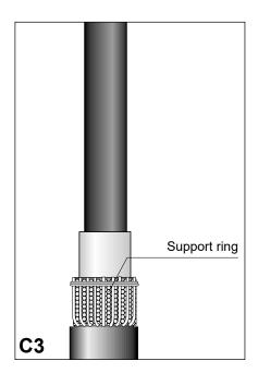
Slide the support ring under the Al wires. Fix the ends of the Al wires with a wire binder onto the support ring.
