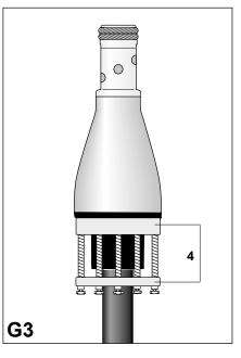
Push the compression device (4) firmly against the silicone stress cone.
