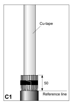
Remove the oversheath and bedding on the reference line.
