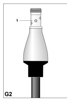
Remove the PVC tape from the conductor.
