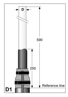
Thoroughly remove the outer semicon layer to within 250 mm above the reference line until the diameter of the insulation is D (see **Table 1**).
