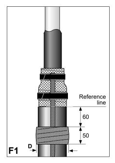
**60 mm below the reference line,** apply a 50 mm wide packing of cotton cloth tape.
