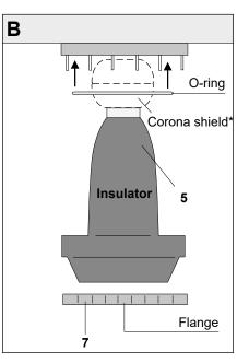
Put the O-ring (supplied by the switchgear/transformer manufacturer) into the sealing groove of the switch gear. Clean and degrease the epoxy insulator (**5**). Keep it free from dust and dirt.
