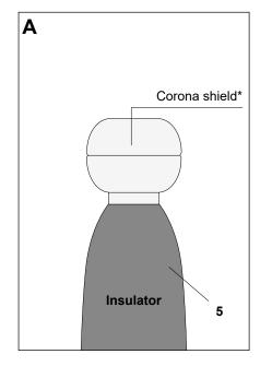
Bolt the lower part of the corona shield to the insulator electrode. Apply the top part of the corona shield.
