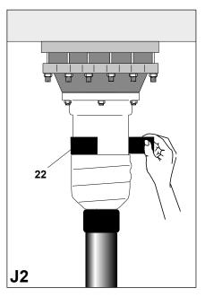
Wrap 1 layer of black mastic (**22**) around the gland above the textile tape.
