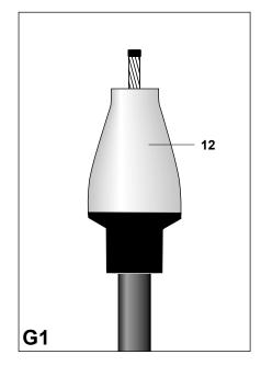
**Installing the silicone stress cone.** Before installing the silicone stress cone (**12**), check it for damages, failure or defects.
