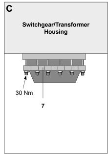
Insert the epoxy insulator (**5**) into the switchgear/transformer housing. Apply the flange (**7**). Bolt the flange evenly to the switchgear/transformer housing.
