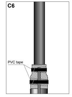
Apply 2 layers of copper mesh to the Al wires and the copper tape.
