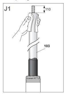
Remove the cable insulation (103) for the length of 110 mm.
