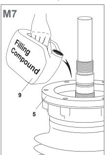
Check the filling level. Make sure the filling compound level is 100 mm below the top of the composite insulator (5).
