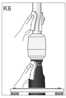
Clean the cable and all parts installed.
