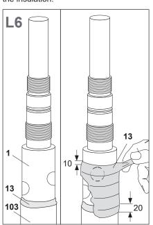
Position the short tube (10) on the lug (1) as shown. Shrink the tube in place starting from the top 10 mm below the edge as shown.
