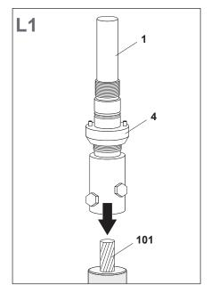
Remove the PVC tape from the conductor (101).
