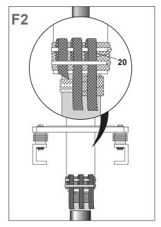
Wrap one contact band (18) around the metal tape and fix it with two to three layers of copper mesh tape (15). Remove the PVC tape and bend down the copper braids (19).
