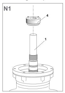
Grease the support nut (4). Slide the support nut over the lug (1).
