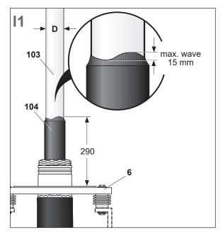
Remove the outer semicon layer (104) to within 290 mm from the base plate (6).
