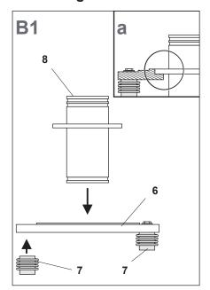
Temporarily fix the support insulators (7) to the base plate (6) with the larger screws.
