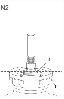
Adjust the support nut (4) temporarily so its surface is flush with the top of the composite insulator (5).
