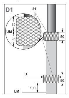
Apply a 50 mm wide packing of textile tape (21) on the upper mark as shown. 100 mm above the lower mark, wrap a second 50 mm wide packing of textile tape starting as shown.
