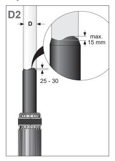
**Chamfer the outer semicon layer** at least 25 - 30 mm.
