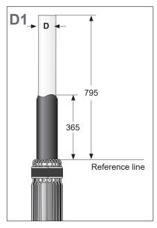
Thoroughly remove the outer semicon layer to within 365 mm above the reference line until the diameter of the insulation is **D** (see **Table 1**).
