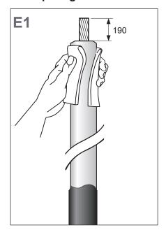
Remove 190 mm of the cable insulation as shown.
