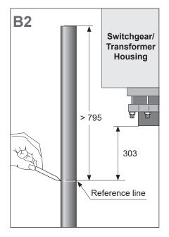
Mark the reference line on the cable 303 mm below the transformer housing as shown.
