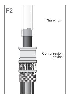
Wrap several layers of plastic foil over the prepared insulation.
