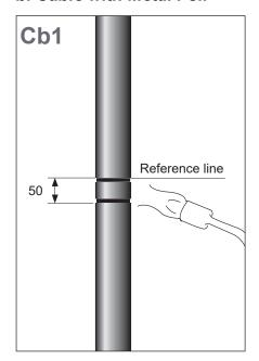
Heat the cable outer jacket (**110**) below the reference line. Soften approx. 50 mm of the surface.
