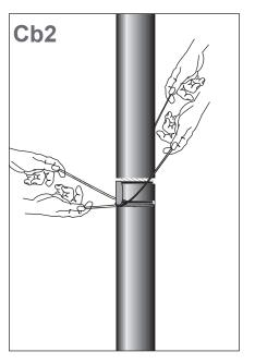
Cut through the outer jacket (110) with the supplied string. Remove the outer jacket from the Al-foil (106) by slicing segments away with the string as shown in the picture.
