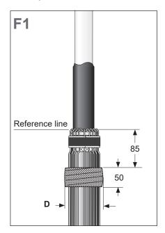
Apply a 50 mm wide packing of textile tape. Start wrapping **85 mm below the reference line** as shown in the drawing.
