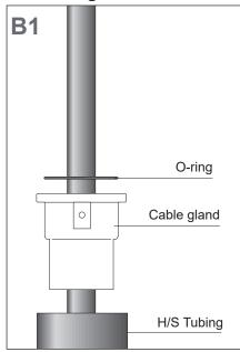
Move the heat shrinkable thick wall tubing, cable gland and O-ring down the cable jacket as shown in the drawing.
