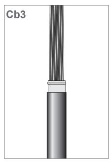
Fix the Al-foil (106) with a wire binder. Clean the Al-foil from traces of the outer jacket (if any). Remove the outer jacket, foil and bedding from the remaining cable end.
