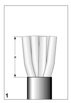
Remove the outer sleeve to dimension **a** as shown in the table. Remove sharp edges, if any.
