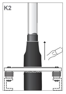
Slide the short heat-shrink tube over the cable down to the base plate and shrink it into place.
