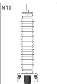
Fix the top plate (3) to the composite insulator (5) as shown in the detail. Use a torque of 50 Nm.
