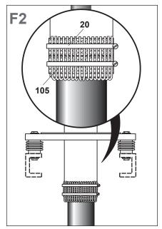
Bend the copper wires (105) back.
