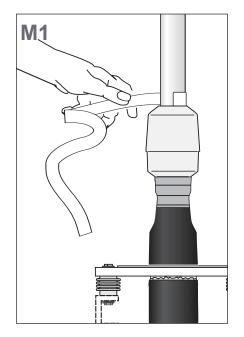
Remove the transparent tape from above the stress cone.
