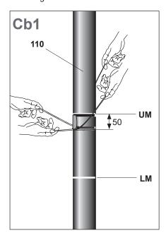
Fix the AL-foil (106) with a wire binder (25). Clean the AL-foil from traces of the outer jacket (if any).
