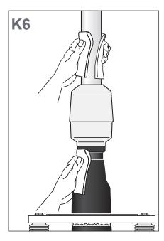
Clean the cable and all parts installed.
