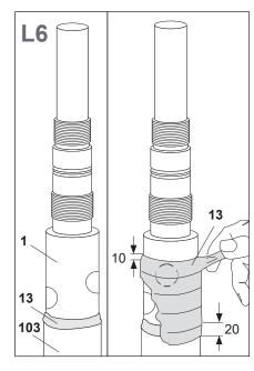
Fill the gap between the lug (1) and the cable insulation (103) with yellow mastic tape (13).
