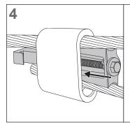
Insert wedge with hardware assembly between conductors. Bracket and bolt may need to be backed out partially to allow for clearance.
