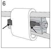
Using impact wrench, drive the bolt to pull back bracket.
