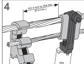
Hook C-body with C-holder over the Main and Tap conductor leaving 6" min. from piggyback clamp.
