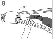
Using appropriate hot stick tool with deep impact socket, insert socket into back of wedge holder to engage bolt head. Drive the bolt using impact wrench to pull back bracket. Ensure bracket hook and tabs lock into place around edges of the C-Body.
