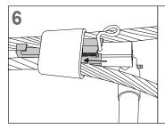
Insert assembly between conductors using universal hot stick. Bracket and bolt may need to be backed out partially to allow for clearance.
