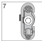
Ensure Main and Tap Conductors are centered in wedge grooves.
