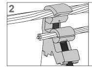
Secure Tap conductor in lower section of piggyback clamp by tightening eye bolt.
