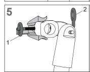
Secure wedge with hardware assembly in wedge holder by firmly tightening locking screw 1 first, then firmly tighten locking screw 2.
