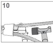
Use rubber end of hammer to loosen the screws and remove wedge holder, leaving wedge in position.
