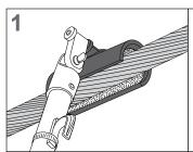
Wire brush Main and Tap conductor with brush attachment on hot stick.
