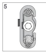
Ensure Main and Tap Conductors are centered in wedge grooves.
