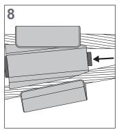
Drive the bolt to fully install the wedge.
