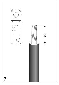
Cut back the insulation according to  $\mathbf{K}$  = depth of cable lug barrel hole.
