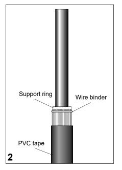
Cut the armour at 60 mm above the sheath cut.
