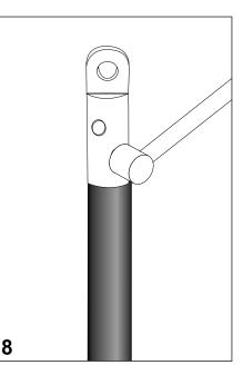
Install the cable lug and remove all sharp edges.
