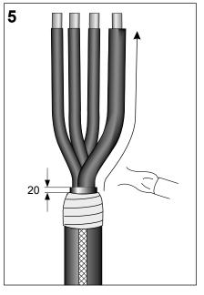
Pass the breakout over the cores and pull it well down into the crutch.
