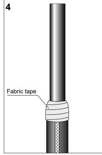
Remove the inner sheath and fillers at 20 mm above the end of armour. Spread and clean the cores.
