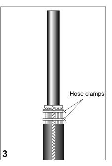
Fix the earth braid over the armour with hose clamps.
