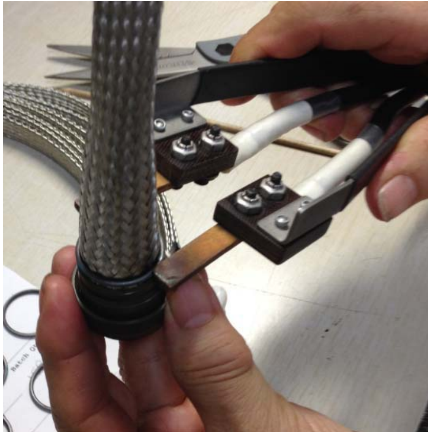
Figure 5 Applying Hand-Tool for Electrical Heating
