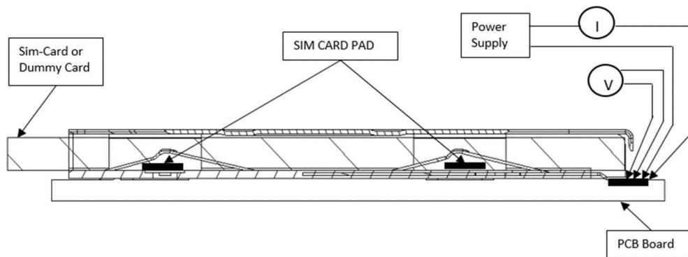
Fig.4 Termination Resistance Measuring Points
