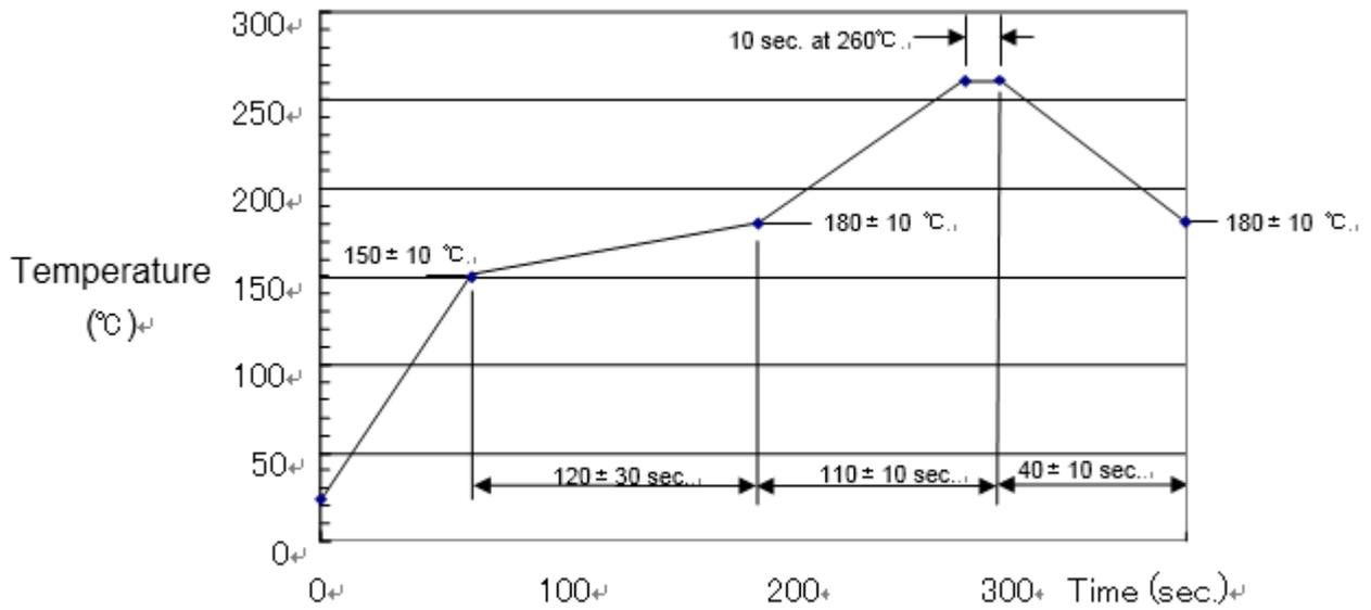
Fig.3 Reflow temperature profile
