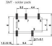
Customer needs to apply enough solder paste volume / thickness / solder material content to ensure a stable solder joint
