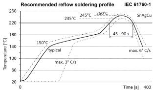
Infrared Soldering: temperature/time profile (lead and housing peak temperature)
