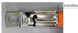
Figure 7: Crimp the ring tongue
