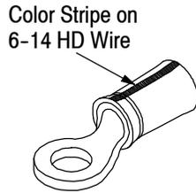
3 Equally Spaced Stripes on Nylon Insulation Restricting
