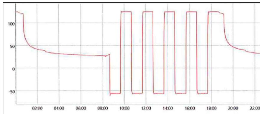
Figure 1 – Thermal Shock Test Chamber Profile
