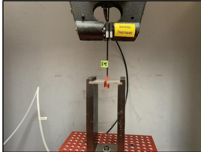
Figure 6 - Tensile Strength Test Setup
