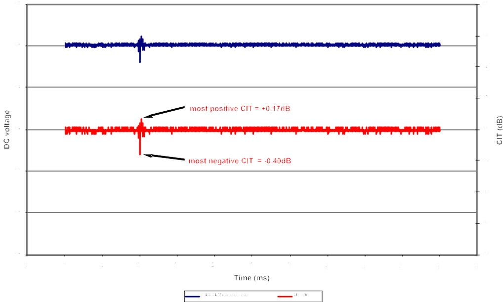
B061295-003 - Transient detected during Random Vibration
