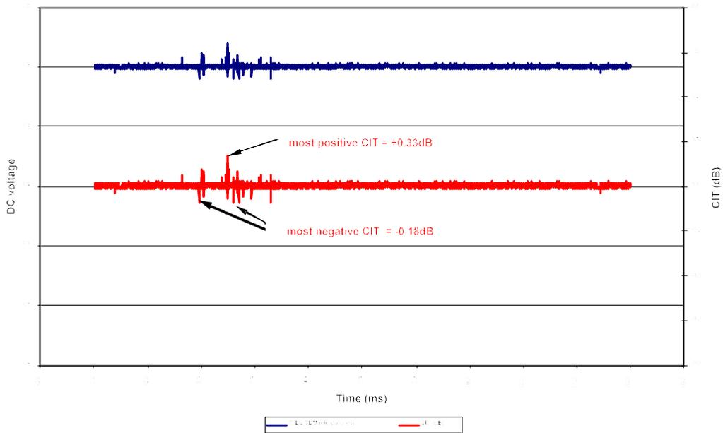
Change in IL and RL after Shock and Vibration Testing
