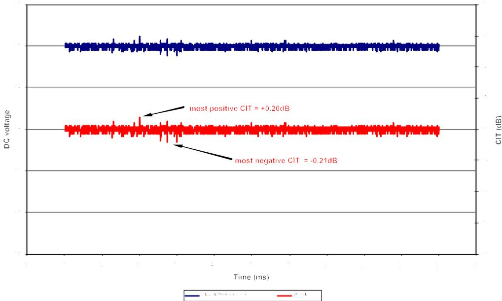
B061295-003 - Worst case transient detected during Sine Vibration
