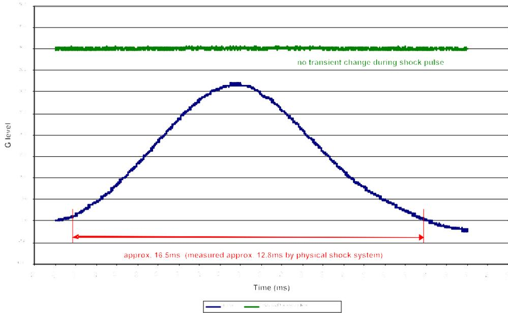
B061295-003 - Physical shock of RWOC SC sample 8 per FOTP-14, Method A (50g, 11ms)
