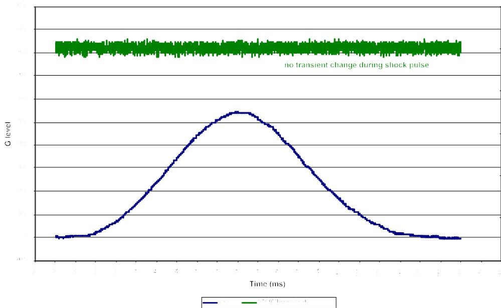
B061295-003 - Physical shock of RWOC SC sample 5 per FOTP-14, Method B (75g, 6ms)
