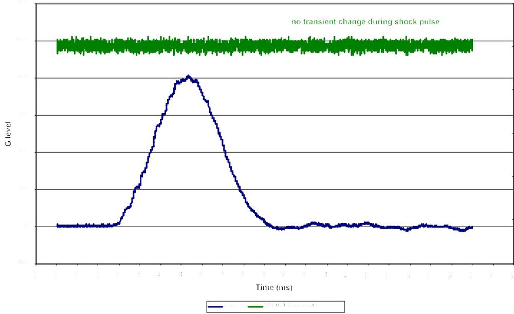
B061295-003 - Worst case transient detected during Mechanical Shock (FOTP-14, Method B, 75g, 6ms) of RWOC LC sample 13
