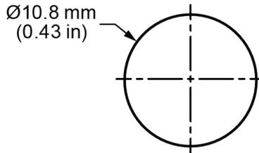
Figure 2. ANT-433-WRT Series Antenna Recommended Enclosure Mounting Dimensions
