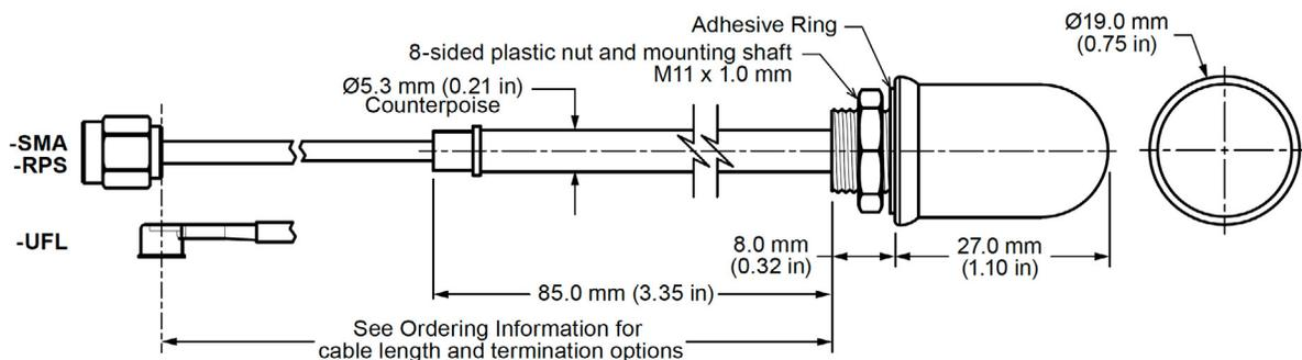
Figure 1. ANT-433-WRT Antenna Dimensions
