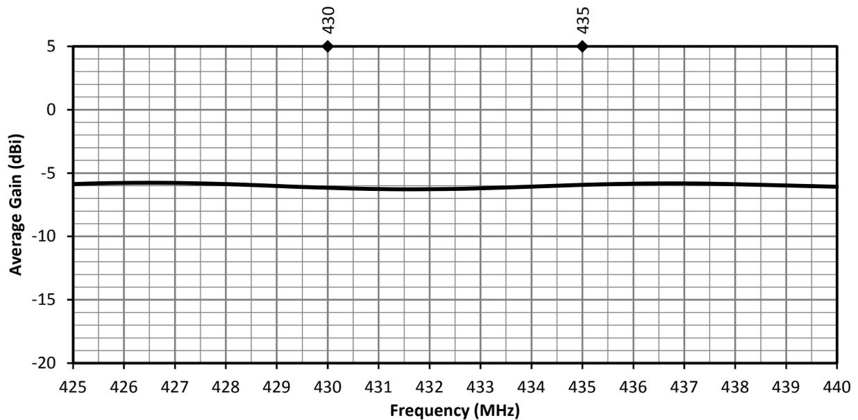
Figure 8. ANT-5GW-MMGI-SMA Antenna Average Gain on Ground Plane
