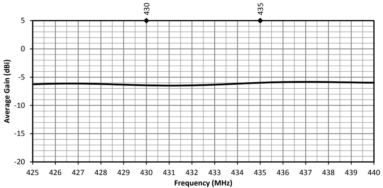
Figure 15. ANT-5GW-MMG1-SMA Antenna Average Gain, Free Space
