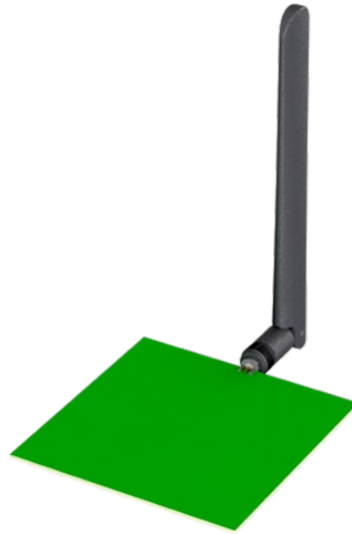
Figure 10. ANT-5GWWS5-SMA on Edge of Ground Plane, Bent 90 Degrees (Edge-Bent)
