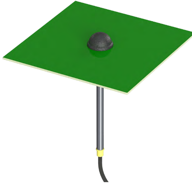
Figure 11. ANT-868-WRT at Center of Ground Plane
