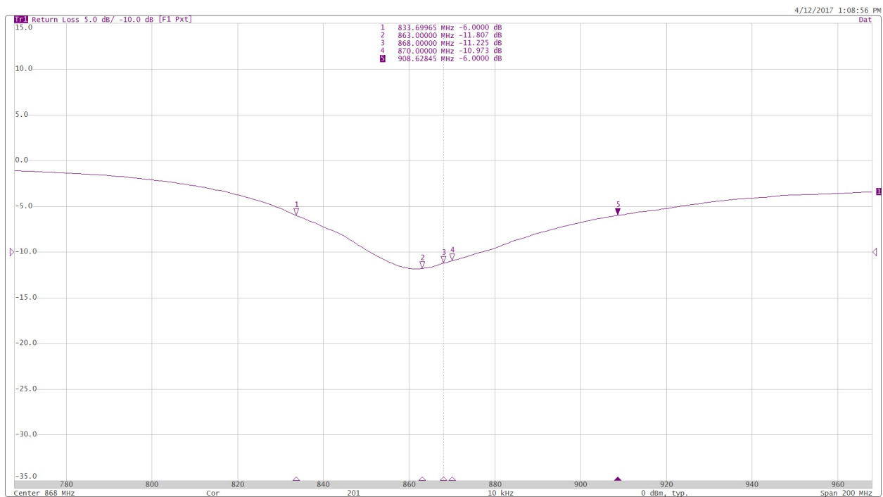
Figure 4: Typical antenna reflection performance
