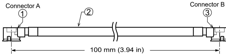
Figure 1. Product Dimensions for the CSG-UFFR-100-UFFR Cable Assembly
