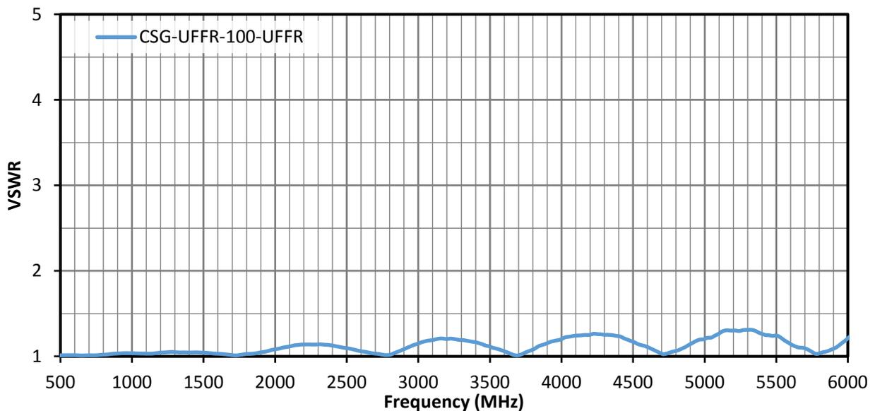
Figure 4. VSWR for the CSG-UFFR-100-UFFR Cable Assemblies
