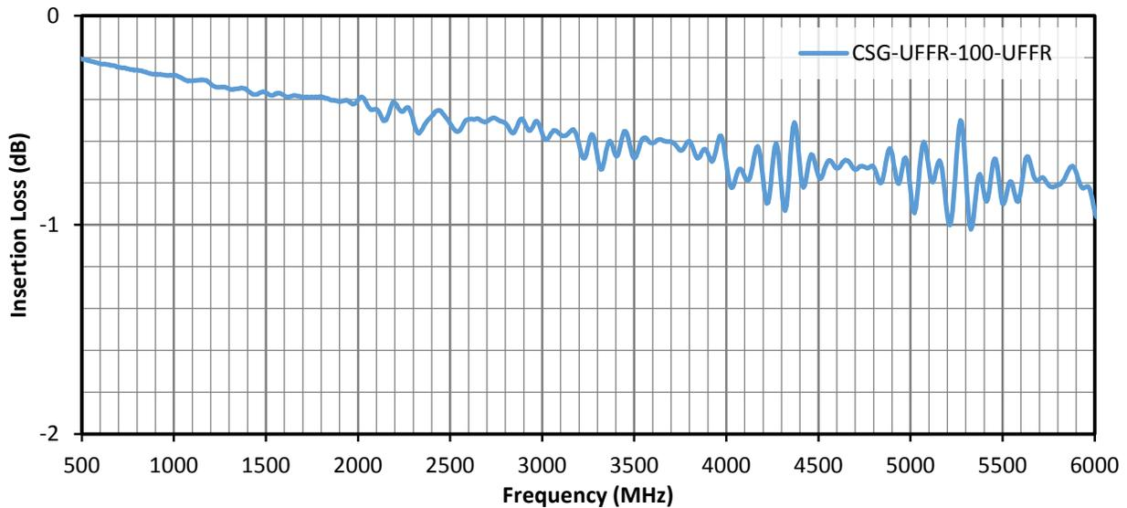
Figure 3. Insertion Loss for the CSG-UFFR-100-UFFR Cable Assemblies
