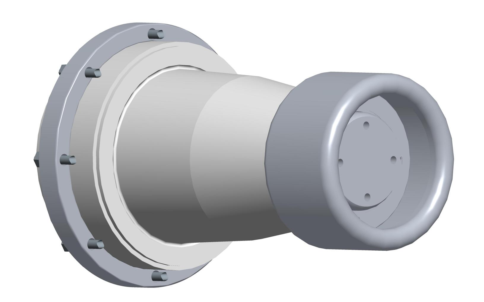
Insulator design according to IEC 62271-209
