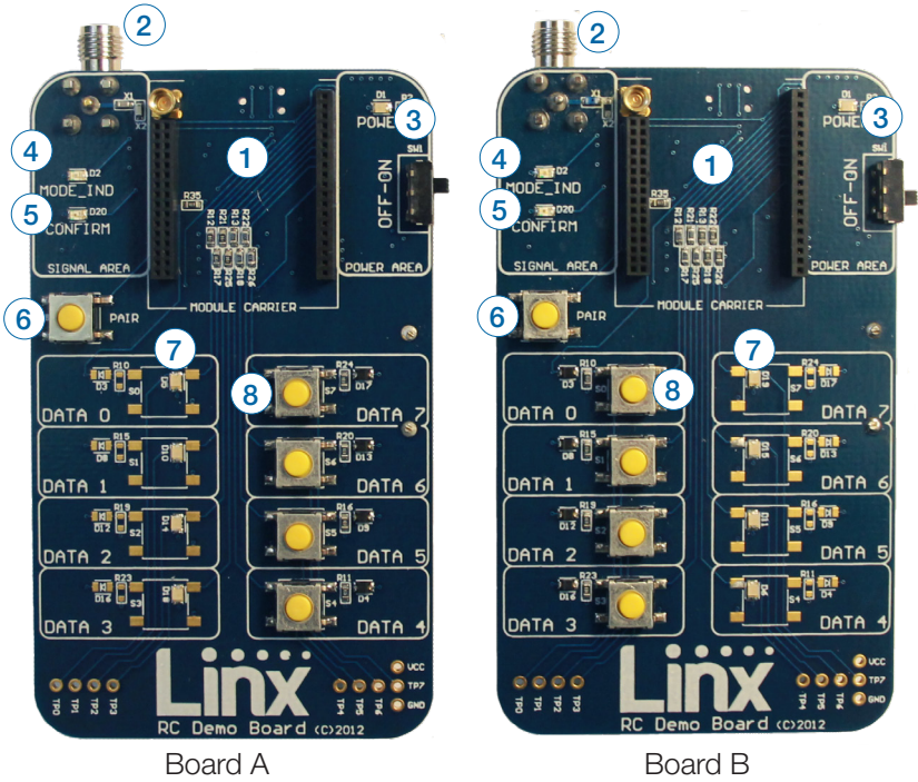
Figure 6: Remote Control Demo Board
