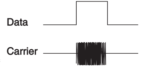
Figure 12: CPCA (AM) Modulation
