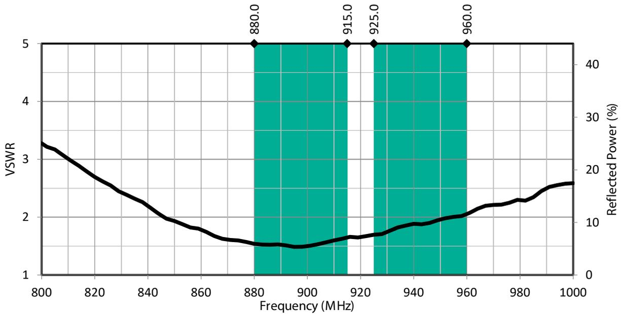
Figure 2: CW LTE Band 8 Antenna Full Bandwidth VSWR
