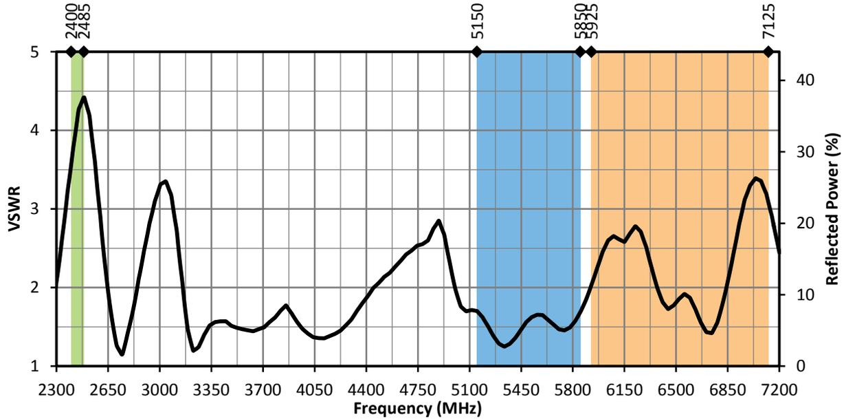
Figure 11. ANT-W63-IPW2-NP Antenna VSWR, Center of Ground Plane
