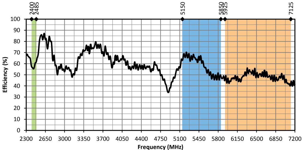
Figure 8. ANT-W63-IPW2-NP Series Antenna Radiation Efficiency, Free Space
