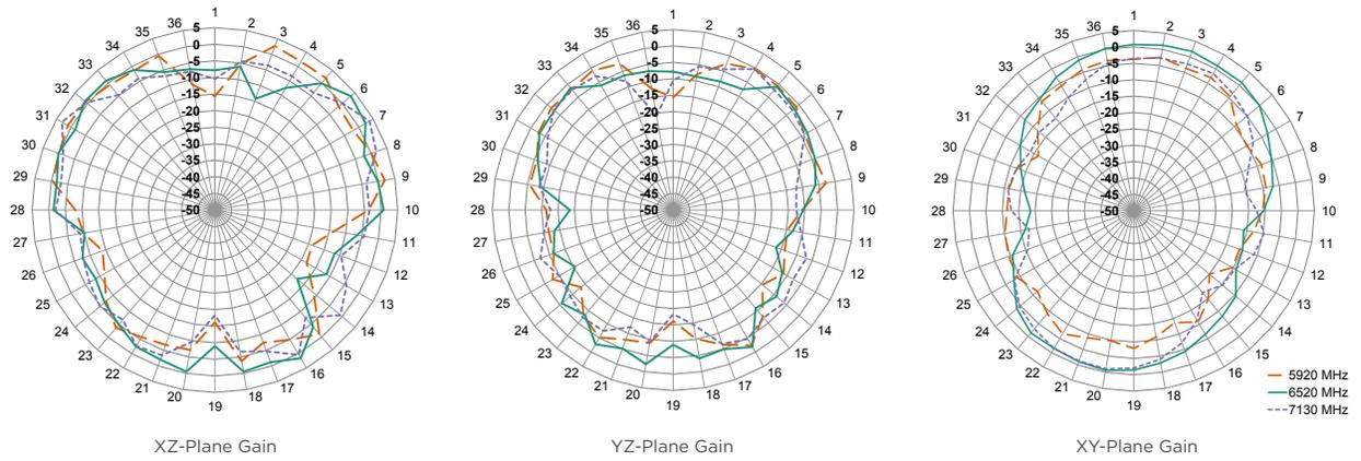
Figure 9. ANT-W63-IPW2-NP Antenna Radiation Patterns, Free Space
