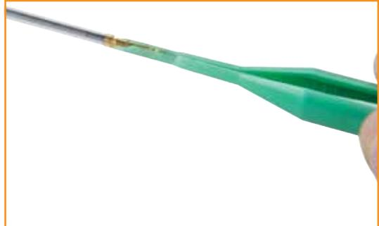
**2** After the wire snaps into the tool, seat the retention shoulder against the tip of the tool.
