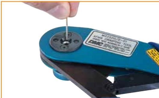
**3** Drop the contact into the crimping tool with the contact crimp barrel facing up.
