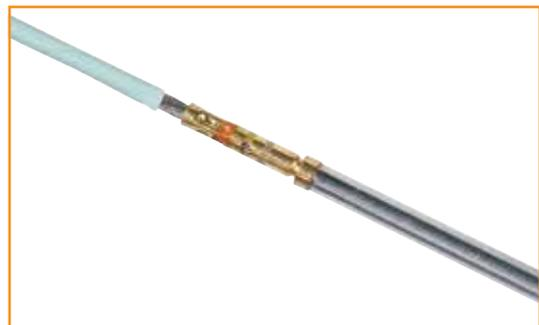
**6** Two series of 4 indents grip the wire and secure the contact to the wire. Visibility of the wire in the contact inspection hole (arrow) indicates that the wire is crimped into the contact at the proper depth. Inspect to make sure there are no loose or nicked strands.
