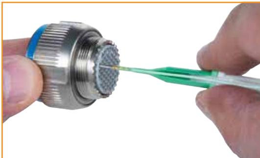
**3** Holding the connector with the rear grommet facing you, slowly push the contact straight into the grommet cavity. Do not twist the tool. Note: Some wire constructions may not require the use of an insertion tool.
