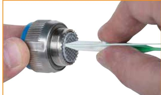
**2** The wire will now have snapped into place. Slide the tool down along the wire and into the rear cavity and slowly into the connector until a positive resistance is felt. At this time, the contact retaining mechanism is in the unlocked position.
