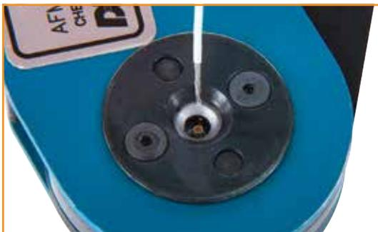
**5** Insert the bare wire into the open end of the contact and squeeze the handles of the tool together. The crimping tool will not release until the full crimping cycle has been performed. Remove the crimped contact and wire from the tool.
