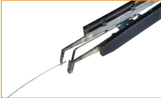
**1** Burn through the insulation with a hot wire stripper or use other approved stripping method. Do not remove the insulation at this point. This will help protect the wire strands from splaying. Refer to contact information sheet for proper wire insulation strip length.
