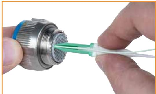
**4** A firm stop will be evident when the contact positively seats in the connector. Remove the tool by sliding it back on the wire. The contact will now be securely locked in place.
