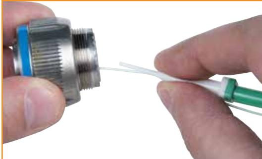
**1** With the rear of the connector facing you, lay the wire of the contact along the slot of the tool, leaving about 1/2" from the end of the tool to the rear of the connector. Squeeze the wire firmly into the tool between the thumb and forefinger about 1/2" from the tip and quickly pull the tool away from the connector.
