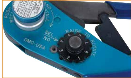
**2** Set the dial of the crimp to the proper setting for wire gage and contact as noted on the contact information sheet or on the tool. Be sure that the proper locator is used. See contact information sheet for proper locator.
