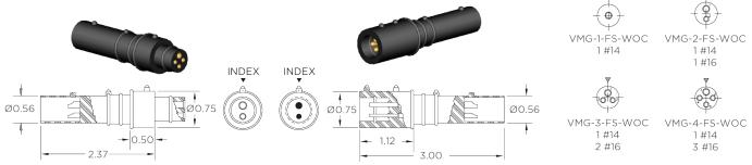
Material: Special Neoprene, Molded Contacts: Copper Alloy, Hard Gold Plated per ASTM-B-488 Voltage: 600 VDC. Contact TE for higher voltage requirements Mated Pressure Rating: Up to 20,000 psi
