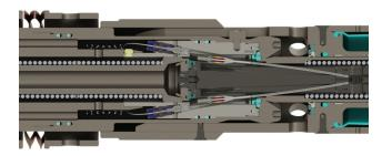
5. Flexible contact guide tubes splay and align via guide-ways in their opposite half, allowing the coupling of the optical ferrules within the benign oil-filled environment.
