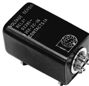
The KILOVAC 1350 series AC voltage sensor energizes a relay when the monitored power line voltage reaches a predetermined level. This rugged unit with reliable solid-state design provides precise, repeatable operation over a wide
