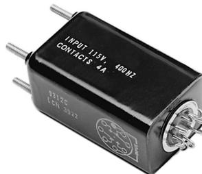
KILOVAC 7000 series frequency sensor utilizes an integrated circuit digital logic design to determine, cycle by cycle, whether a given input signal is within a predetermined frequency pass band. Typical application is in monitoring MIL-STD-704 power systems.
