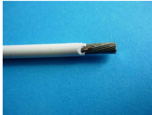
NOT ACCEPTABLE Damaged and Nicked Conductors
