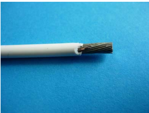
NOT ACCEPTABLE Insulation not cut cleanly
