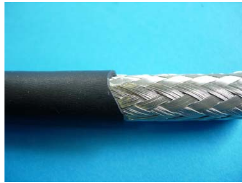
NOT ACCEPTABLE Insulation not cleanly cut
