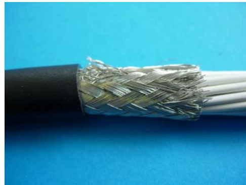
NOT ACCEPTABLE Shield strands damaged
