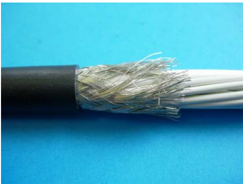
NOT ACCEPTABLE Shield opened up
