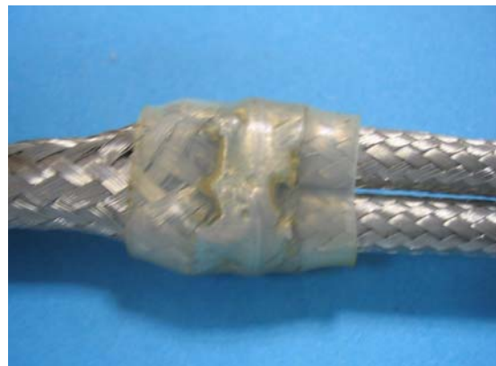
Figure 5B Insufficient Solder Flow
