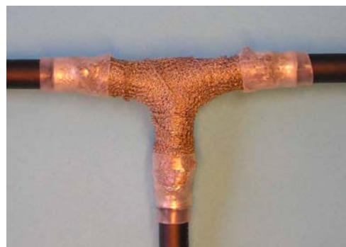
NOT ACCEPTABLE Poor wrapping of tape and Shield spike through insulation
