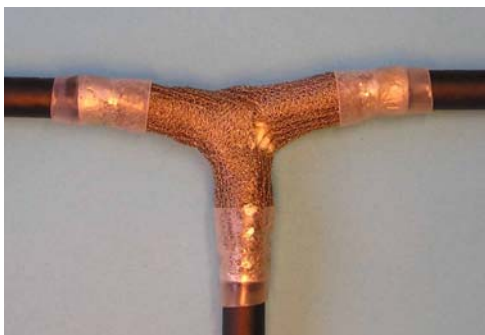
NOT ACCEPTABLE Weave of shield open
