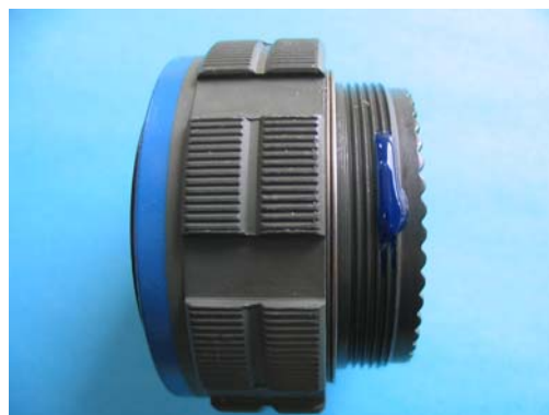
ACCEPTABLE Loctite™ positioned on the first 2 to 3 threads
