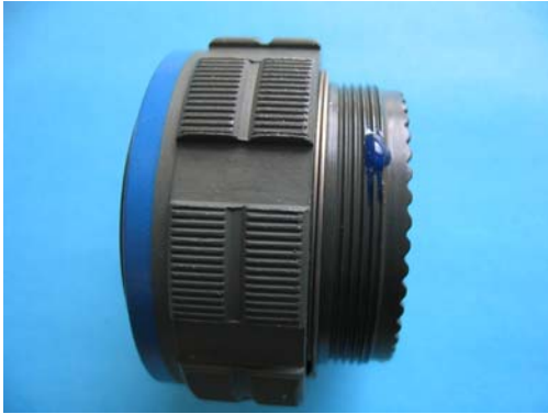
NOT ACCEPTABLE Insufficient Loctite™ applied
