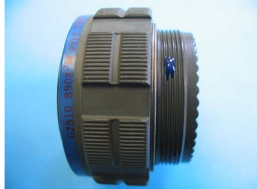
NOT ACCEPTABLE Loctite™ applied to incorrect position, must be first 2/3 threads
